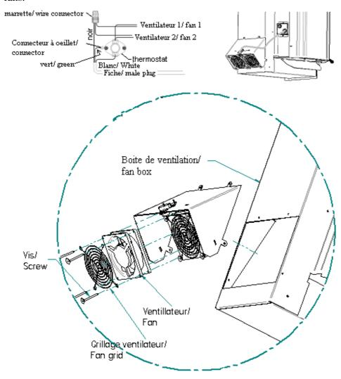
The electrical cord of the fans must never touch the appliance surfaces or pass under the appliance in order to avoid electrical shock or fire.
