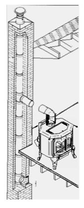
The *Vulcain* wood appliance must be installed in accordance with the applicable local laws or the CAN/CSA - B365 ULC S635, ULC S640, UL 1777 norms. Install the chimney following the manufacturer's instructions.
