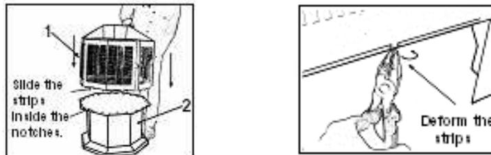
2. Assemble the chimney in one piece and slide the hat on the conic part of the chimney and then screw it into the 2 holes at the bottom of the hat. Lift up the 4 clips located in the hole of the top at 90 degrees. Place the chimney between these 4 clips and screw them on the chimney with 4 screws.
