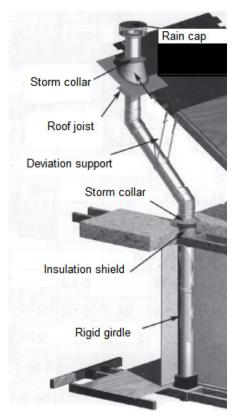
The *Olympien* central fireplace must be installed in accordance with the applicable local laws or the CAN/CSA – B365 NFPA211 (USA) norms. For the chimney, follow the chimney manufacturer's instructions.
