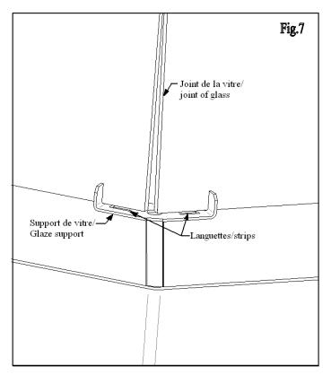
To straighten the glass joint, lift up the strips with a slotted screwdriver. (fig.8)
