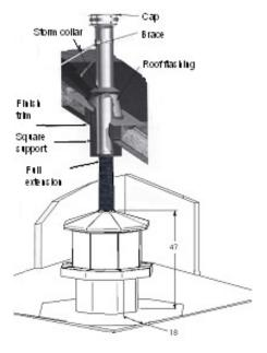
The *Olympien* central fireplace must be installed in accordance with the applicable local laws or the CAN/CSA – B365 NFPA211 (USA) norms. For the chimney, follow the chimney manufacturer's instructions.
