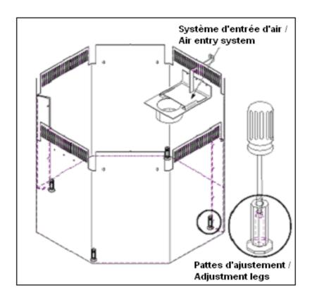
Put your fireplace at the desired location and verify the level. If the base is not levelled, use a slotted screwdriver to screw or unscrew the legs of the fireplace until it is levelled.
