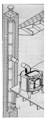
The *Oasis* wood appliance must be installed in accordance with the applicable local laws or the ULC S635, ULC S640, NFPA211 (USA) norms. Install the chimney following the manufacturer's instructions.
