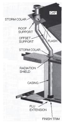
The *Oasis* wood appliance must be installed in accordance with the applicable local laws or the CAN/CSA-B365, NFPA211 (USA) norms. Install the chimney following the manufacturer's instructions.
