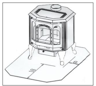
You must install a fireproof plate under the appliance, which must exceed it of 18 inches at the front, of 8 inches at the sides and of 8 inches at the back.
