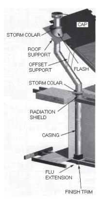
The *Oasis* wood appliance must be installed in accordance with the applicable local laws or the CAN/CSA-B365, NFPA211 ( USA ) norms. Install the chimney following the manufacturer's instructions.
