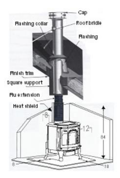
The *Oasis* wood appliance must be installed in accordance with the applicable local laws or the CAN/CSA-B365, NFPA211 ( USA ) norms. Install the chimney following the manufacturer's instructions.
