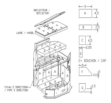
Install the firebricks on the sides and then, the ones on the back of the appliance. To finish with, put the firebricks of the top.
