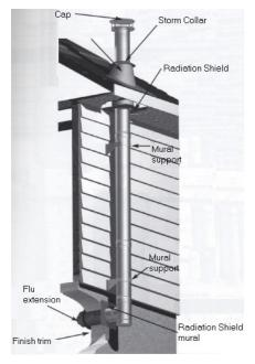
The *Oasis* wood appliance must be installed in accordance with the applicable local laws or the CAN/CSA-B365, NFPA211 (USA) norms. Install the chimney following the manufacturer's instructions.
