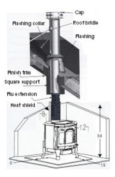
The *Oasis* wood appliance must be installed in accordance with the applicable local laws or the CAN/CSA-B365, NFPA211 (USA) norms. Install the chimney following the manufacturer's instructions.
