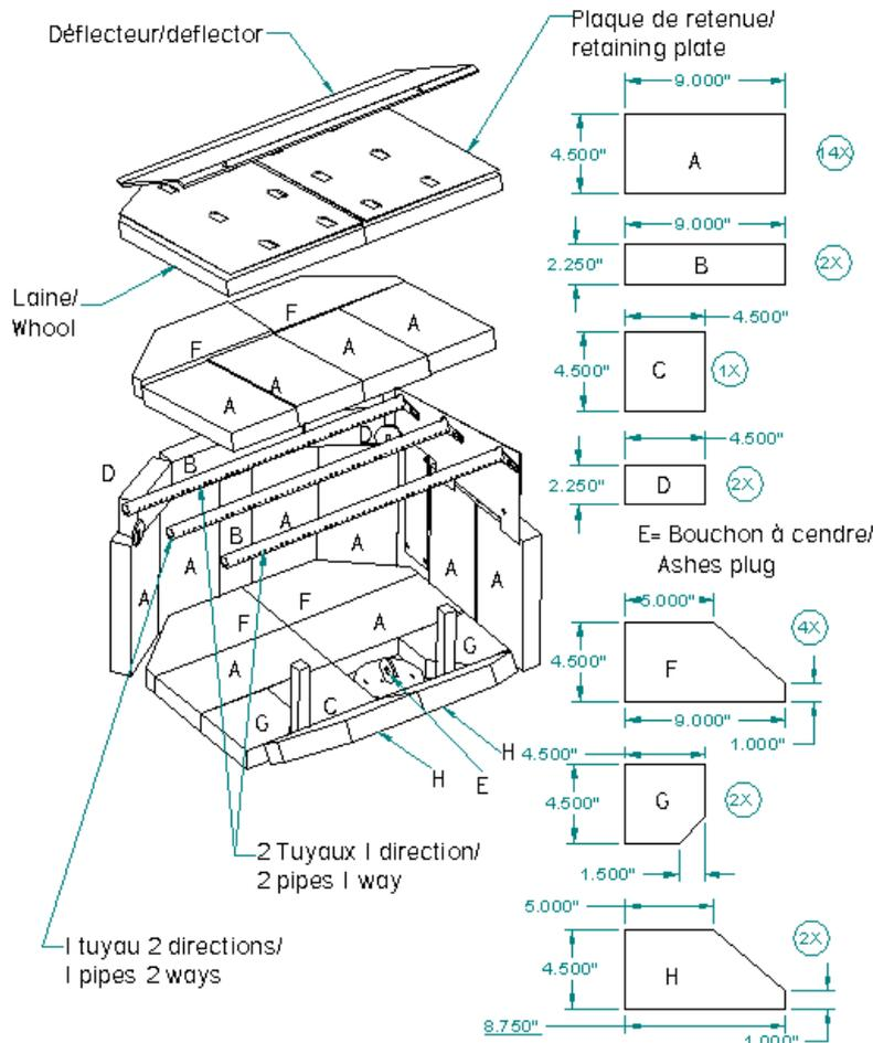
Place the firebricks as illustrated. They are identified by the letters **A** to **H** and the seal cap is identified by the letter **E**.
