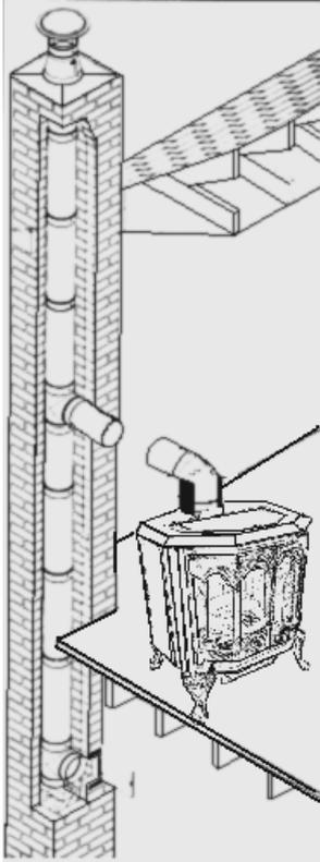
The *Mystere* wood appliance must be installed in accordance with the applicable local laws or the ULC S635, ULC S640, NFPA211 ( USA ) norms. Install the chimney following the manufacturer's instructions.
