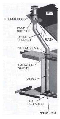
The *Mystere* wood appliance must be installed in accordance with the applicable local laws or the CAN/CSA-B365, NFPA211 ( USA ) norms. Install the chimney following the manufacturer's instructions.
