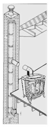
The *Mystere* wood appliance must be installed in accordance with the applicable local laws or the ULC S635, ULC S640, NFPA211 ( USA ) norms. Install the chimney following the manufacturer's instructions.
