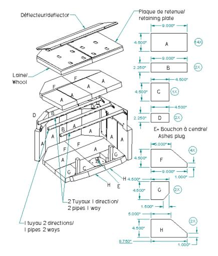
Place the firebricks as illustrated. They are identified by the letters **A** to **H** and the seal cap is identified by the letter **E**.
