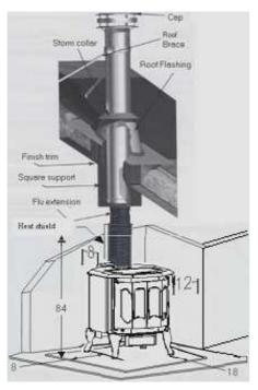
The *Mystere* wood appliance must be installed in accordance with the applicable local laws or the CAN/CSA-B365, NFPA211 ( USA ) norms. Install the chimney following the manufacturer's instructions.
