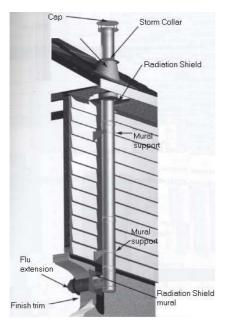
The *Mystere* wood appliance must be installed in accordance with the applicable local laws or the CAN/CSA-B365, NFPA211 ( USA ) norms. Install the chimney following the manufacturer's instructions.
