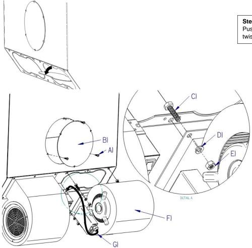
**Step 1 :** Remove the bottom right plate. Push on one side of the plate to tilt it. Keep twisting the plate until it comes apart.
