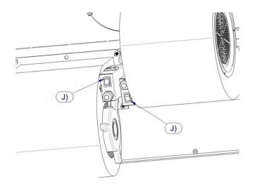
It is possible to change the speed of the blower(s) in between the high and the low speed. The position of the switch(es) as shown in the adjacent picture (J) should correspond to the low speed configuration. **Note:** There is no off position on the switch(es)
