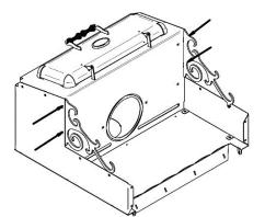
6) Attach the top part to the back and the front.
