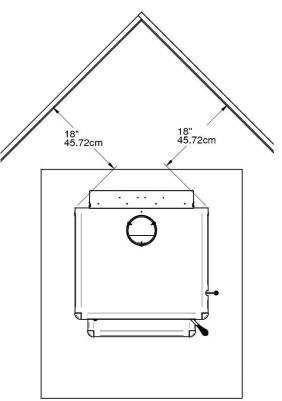
• For a 45° corner installation, or other corner installation, the minimum clearance between the cook stove and combustible material must be 18 inches.
