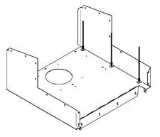
4) Attach the front part (with the door) to the two sides and the back. Leave the horizontal holes empty for the chrome decoration.
