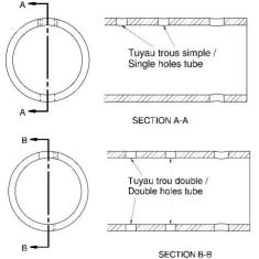
To make sure of right orientation of tube, you find a notch at one end of tubes. The holes on the air intake passage are made into corresponding shapes.
