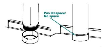
WARNING: It is mandatory to screw the pipe to the stove collar and also at each joints with a minimum of 3 screws.
