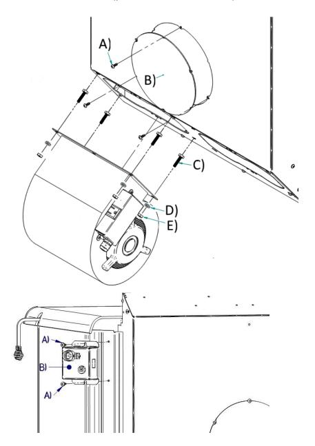
Step 1 : Remove the access panel (B) on the back of the appliance by unscrewing / untightening the 3 screws (A). Insert the 4 bolts (C) inside the fan housing at the designated location by passing the hand through the access opening. Take care of putting the bolt's screwing part oriented downward. Fastened the fan to the stove with the 4 lock washers (D) and the 4 nuts (E) provided with the fan kit as shown hereby
