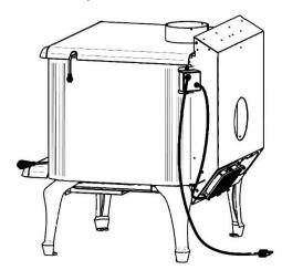
1) Install the two fans at the bottom of vent box as illustrated. Please note that the cords must be placed as shown.
