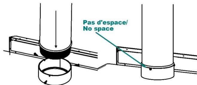
4. Install all the next section up to the roof chimney support and screw every chimney connector parts with 3 screws
