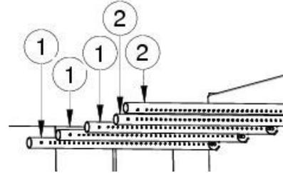
The 2 tubes in front of the heat chamber are double-side perforated tube (2).
