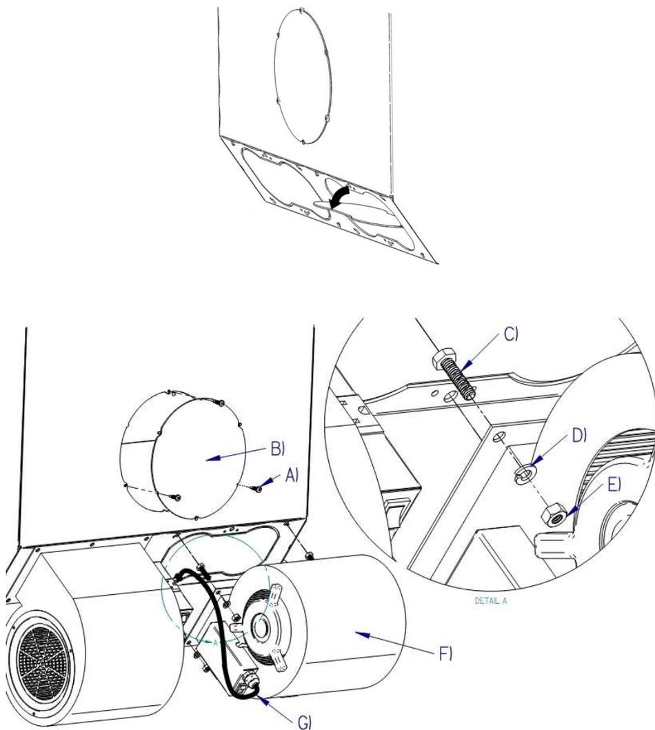
**Step 1 :** Remove the bottom right plate. Push on one side of the plate to tilt it. Keep twisting the plate until it comes apart.
