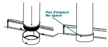
WARNING: It is mandatory to screw the pipe to the stove collar and also at each joint with a minimum of 3 screws.
