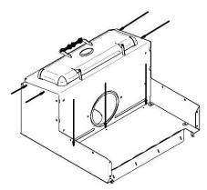
5- Insert the chrome decoration in the holes and fix it with carriage bolts and nuts (with 2 bolts each).
