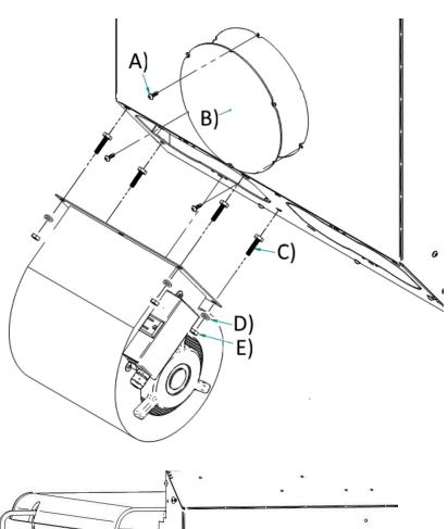
Step 1: Remove the access panel (B) on the back of the appliance by unscrewing / untightening the 3 screws (A). Insert the 4 bolts (C) inside the fan housing at the designated location by passing the hand through the access opening. Take care of putting the bolt's screwing part oriented downward. Fastened the fan to the stove with the 4 lock washers (D) and the 4 nuts (E) provided with the fan kit as shown hereby
