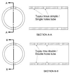
To make sure of right orientation of tube, you find a notch at one end of tubes. The holes on the air intake passage are made into corresponding shapes.
