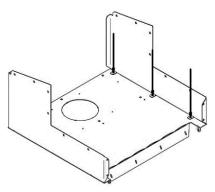
4- Attach the front part (with the door) to the two sides and the back. Leave the horizontal holes empty for the chrome decoration.
