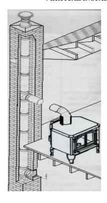
The *Atmosphere EPA* must be installed in accordance with the applicable local laws or the CAN/CSA - B365 ULC S635, ULC S640 norms. For the chimney, follow the chimney manufacturer's instructions.
