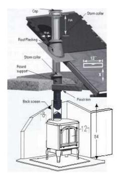
The *Atmosphere EPA* must be installed in accordance with the applicable local laws or the CAN/CSA - B365 ULC S635, ULC S640 norms. For the chimney, follow the chimney manufacturer's instructions.
