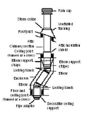
The *ATFM* wood appliance must be installed in accordance with the applicable local laws or the CAN/CSA-B365 norm. Install the chimney following the manufacturer's instructions.
