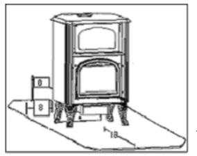
You must install a fireproof plate under the appliance, which must exceed it of 18 inches at the front, of 8 inches at the sides and of 8 inches at the back.
