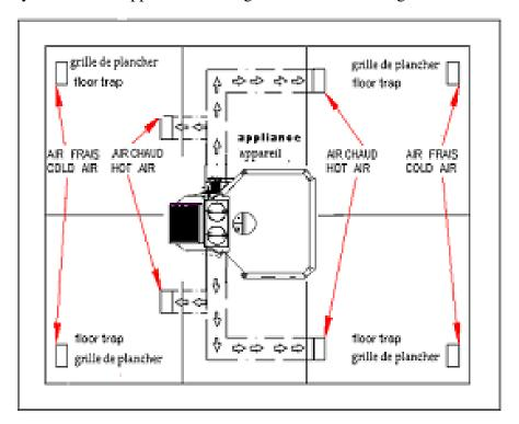
It is recommended to install a floor trap in order to balance the air pressure between the floor where the appliance is installed and the superior floor.
