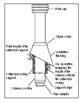
The *ATFM* wood appliance must be installed in accordance with the applicable local laws or the CAN/CSA-B365 norm. Install the chimney following the manufacturer's instructions.
