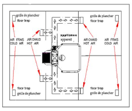
It is recommended to install a floor trap in order to balance the air pressure between the floor where the appliance is installed and the superior floor.
