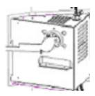
3) To measure out the quantity of air into the combustion chamber, you have to rotate the handle.; upwards for an opening and downwards for a closing.
