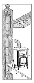
The *ATFM* wood appliance must be installed in accordance with the applicable local laws or the CAN/CSA-B365, ULC S635, ULC S640, UL 1777 norms. Install the chimney following the manufacturer's instructions.
