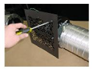
Screw the fan grid (GV460) by using 5 bolts (1" X 1/4") with locks.
