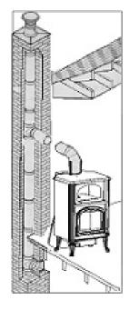
The *ATFM* wood appliance must be installed in accordance with the applicable local laws or the CAN/CSA-B365, ULC S635, ULC S640, UL 1777 norms. Install the chimney following the manufacturer's instructions.
