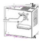
3) To measure out the quantity of air into the combustion chamber, you have to rotate the handle.; upwards for an opening and downwards for a closing.
