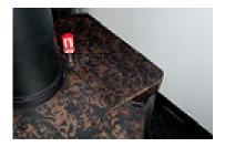
➤ Be sure that the panel recovering the two 6 inches exits over the appliance is well closed and fixed.
