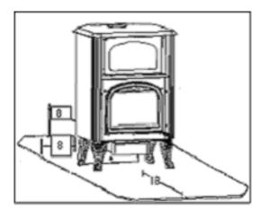
You must install a fireproof plate under the appliance, which must exceed it of 18 inches at the front, of 8 inches at the sides and of 8 inches at the back.
