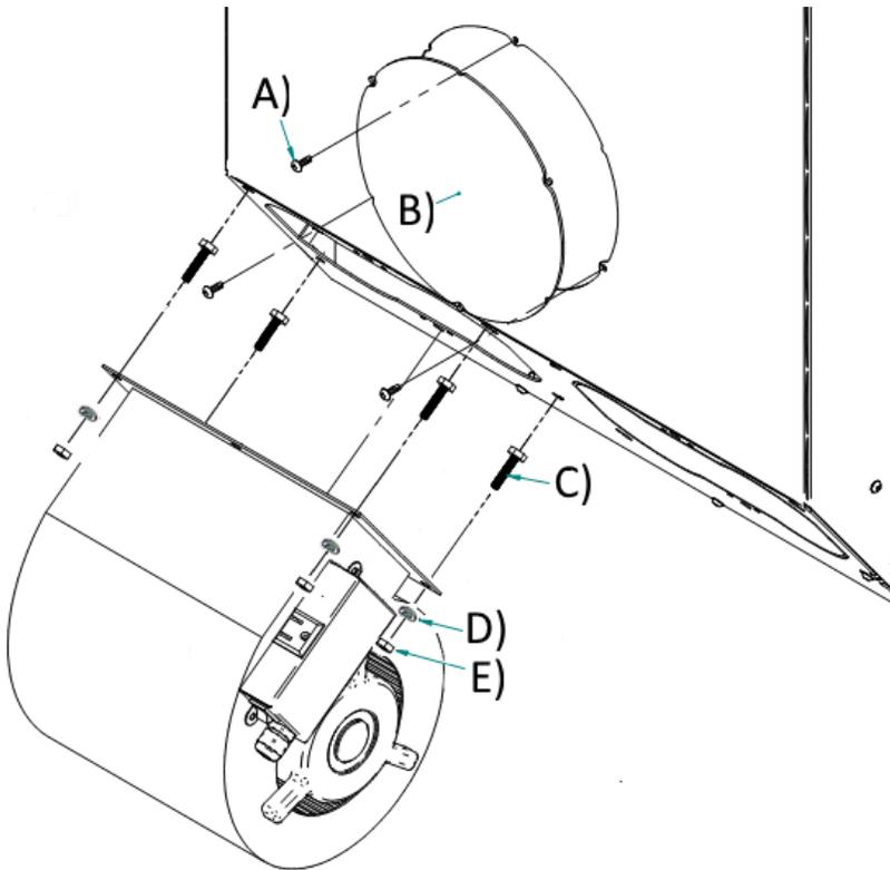
**Step 2:** Install the fan kit's thermodisk junction box (B) by screwing it to the appliance with 2 screws (A) (included). The thermodisk junction box should be located on the back corner of the stove as in the hereby picture . Connect the power cable plug of the thermodisk junction box to the power supply.
