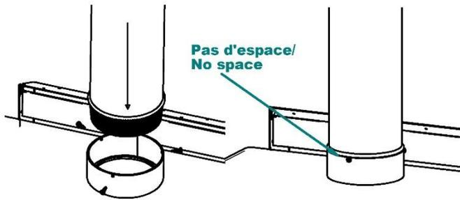
**WARNING: It is mandatory to screw the pipe to the stove collar and also at each joints with a minimum of 3 screws.**
