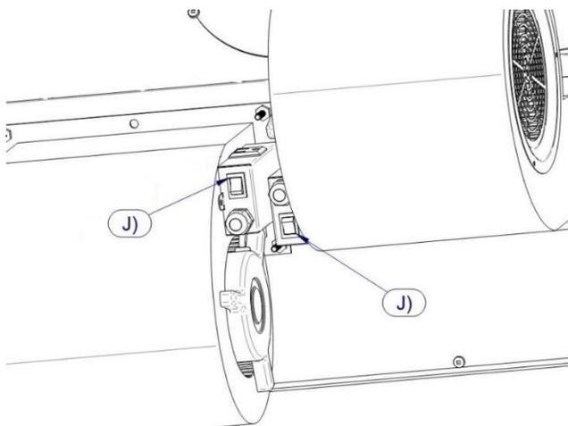
It is possible to change the speed of the blower(s) in between the high and the low speed. The position of the switch(es) as shown in the adjacent picture (J) should correspond to the low speed configuration.
