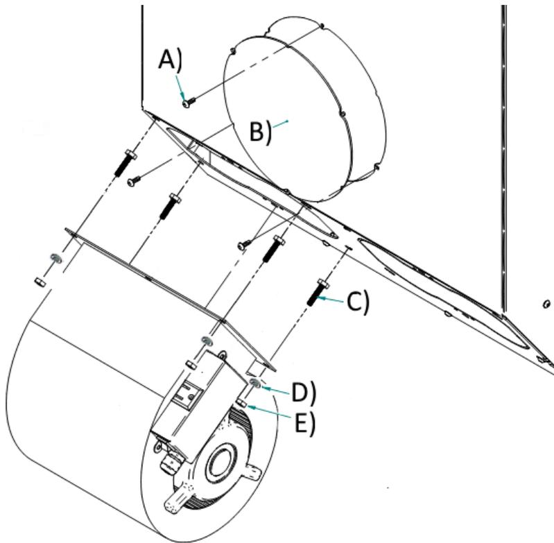
**Step 1 :** Remove the access panel (B) on the back of the appliance by unscrewing / untightening the 3 screws (A). Insert the 4 bolts (C) inside the fan housing at the designated location by passing the hand through the access opening. Take care of putting the bolt's screwing part oriented downward. Fastened the fan to the stove with the 4 lock washers (D) and the 4 nuts (E) provided with the fan kit as shown hereby
