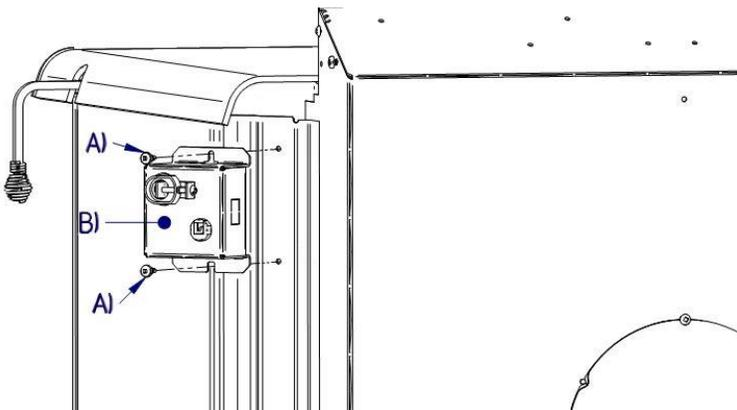
**Step 2:** Install the fan kit's thermodisk junction box (B) by screwing it to the appliance with 2 screws (A) (included). The thermodisk junction box should be located on the back corner of the stove as in the hereby picture. Connect the power cable plug of the thermodisk junction box to the power supply.
