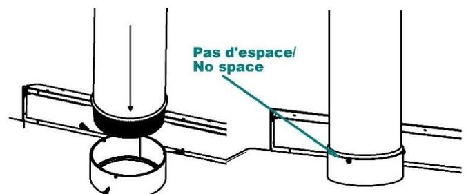
**WARNING: It is mandatory to screw the pipe to the stove collar and also at each joint with a minimum of 3 screws.**
