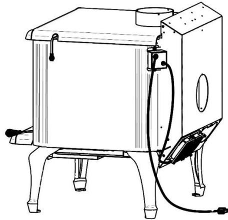
1. Install the two fans at the bottom of vent box as illustrated. Please note that the cords must be placed downward.
